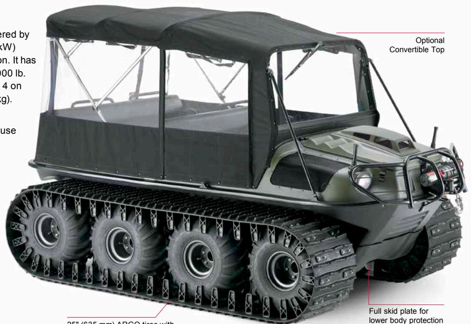
25" (635 mm) ARGO tires with proprietary tread design shown with optional rubber tracks
