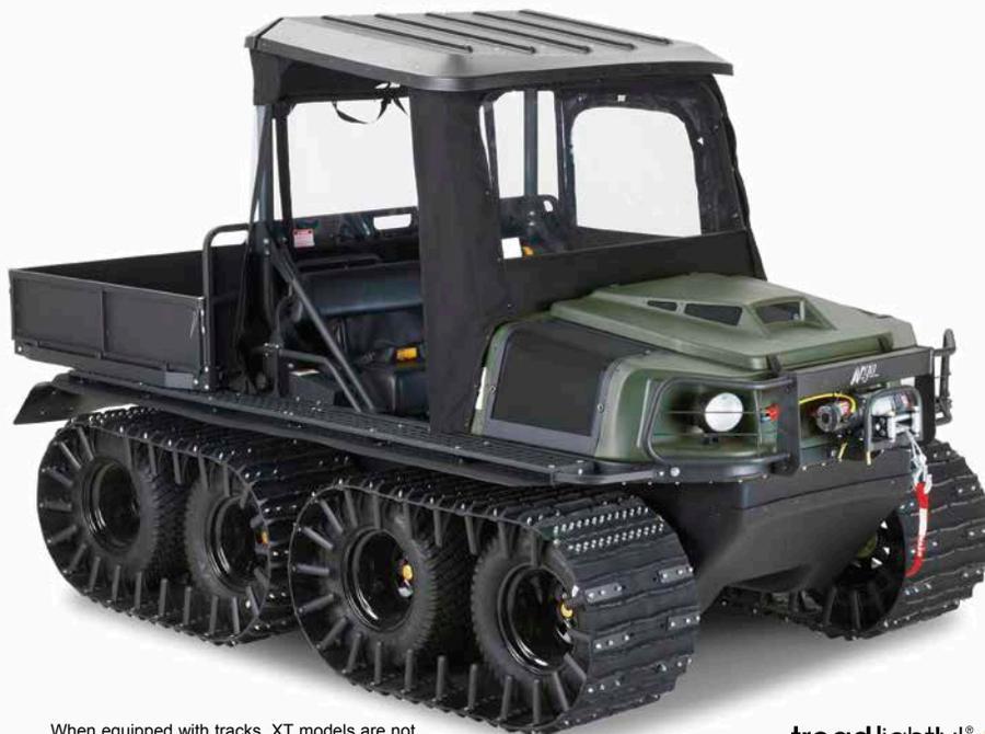
When equipped with tracks, XT models are not fully amphibious, however water crossing is possible with a fording depth of 26" (660 mm).
