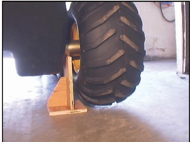
*Figure 9-1. Correct placement of blocks*
