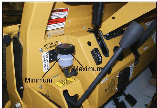
Figure 7-15. Remote translucent master cylinder well.
