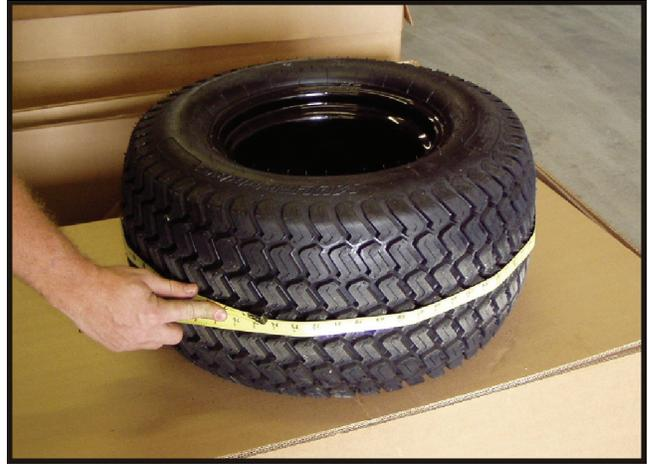
Figure 11-1. Measuring the tire.
